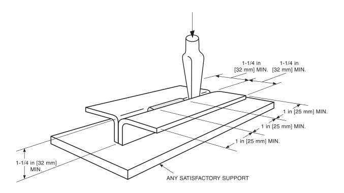
Figure 4.3C—Test for Flare-V-Groove Welds [see 4.6.3.2(2)(b)]
