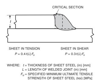
Figure C-2.2—Load Capacity of Fillet Welds
