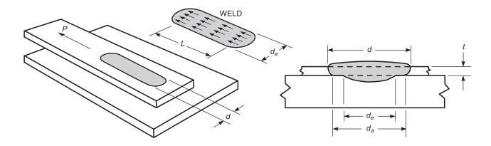
Figure C<u>-2.4</u>—Arc Seam Weld in a Supporting Plate
