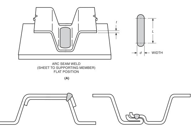
(B) CROSS SECTIONS OF ARC SEAM WELDS
