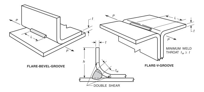
Figure 2.3C—Double-Shear in Flare-Groove Welds [see 2.2.3(2)]
