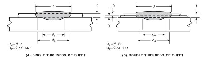
Figure 2.4—Arc Spot Welds (see 2.2.4)
