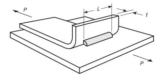
Figure 2.3A—Single-Flare-Bevel-Groove Weld [see 2.2.3(1)]
