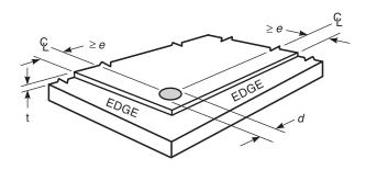
Figure 2.11A—Edge Distances for Arc Spot Welds (see 2.3.5.2)
