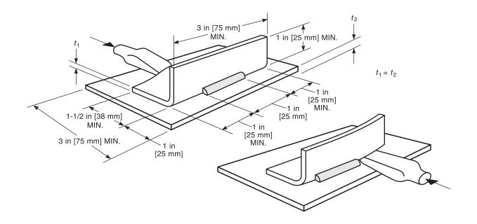
Figure 4.3A—Test for Sheet to Sheet Flare-Bevel-Groove Welds [see 4.6.3.2(1)(a)]
