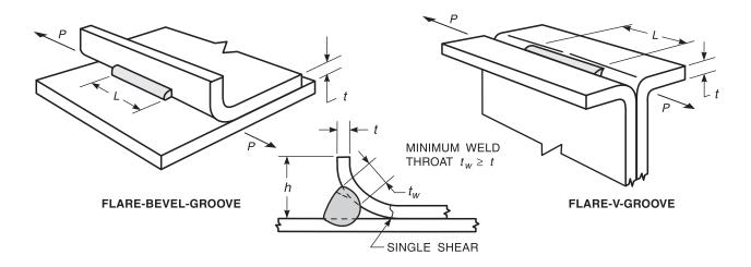
Figure 2.3B—Single-Shear in Flare-Groove Welds [see 2.2.3(2)]
