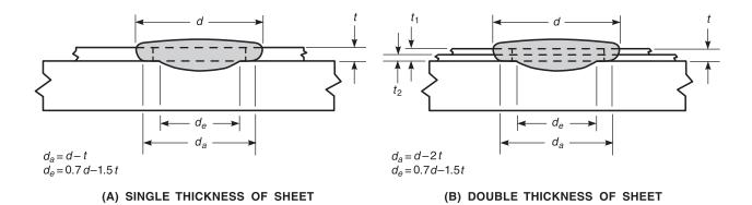
Figure 2.6—Arc Plug Welds (see 2.2.6)
