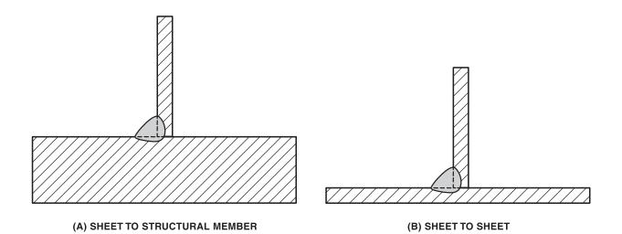
Figure 2.8—Fillet Welds in T-Joints (see 2.3.3.2)
