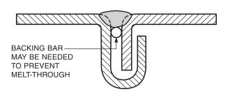
Figure 2.10—Single-Flare-V-Groove Weld (see 2.3.4.2)
