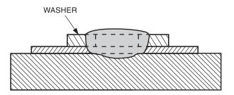
Figure 2.11B—Arc Spot Weld Using Washer (see 2.3.5.3)
