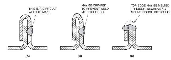
Figure 2.12—Arc Seam Welds Along Standing Rib (see 2.2.5)
