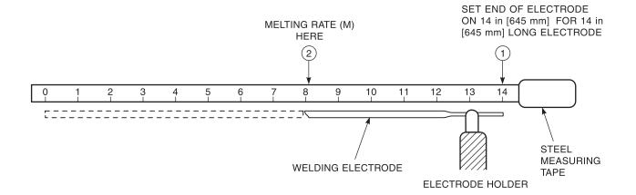
Figure C-4.1—Melting Rate Measurement Illustrated
