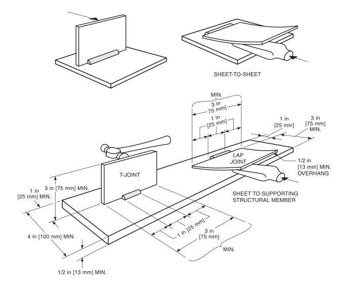
Figure 4.2A—Test for Fillet Welds [see 4.6.2.2(1)]
