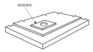
Figure 2.11C—Typical Weld Washer (see 2.3.5.3)
