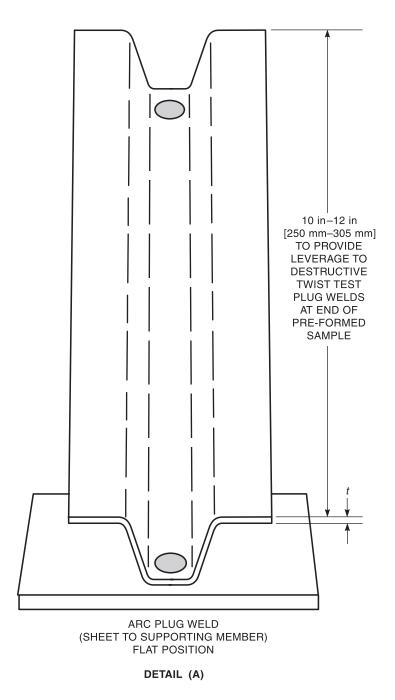
Typical for multi-ply sheet to supporting structural member or sheet-to-sheet—also used for horizontal, vertical, and overhead positions.
